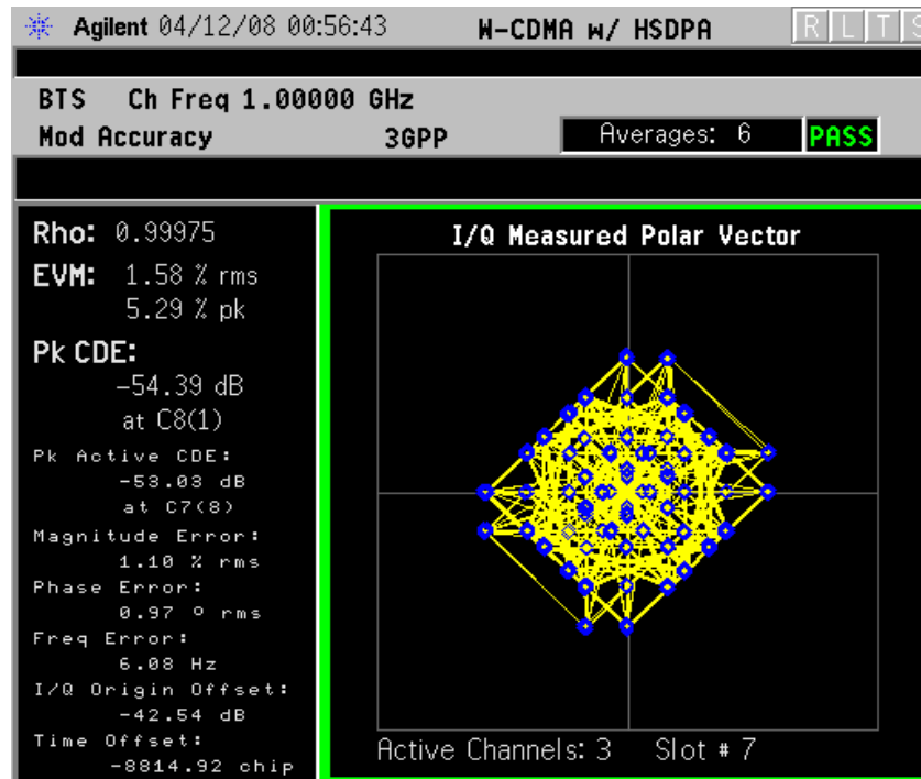
Figure 3-14 Modulation Accuracy Measurement - I/Q Measured Polar Graph
