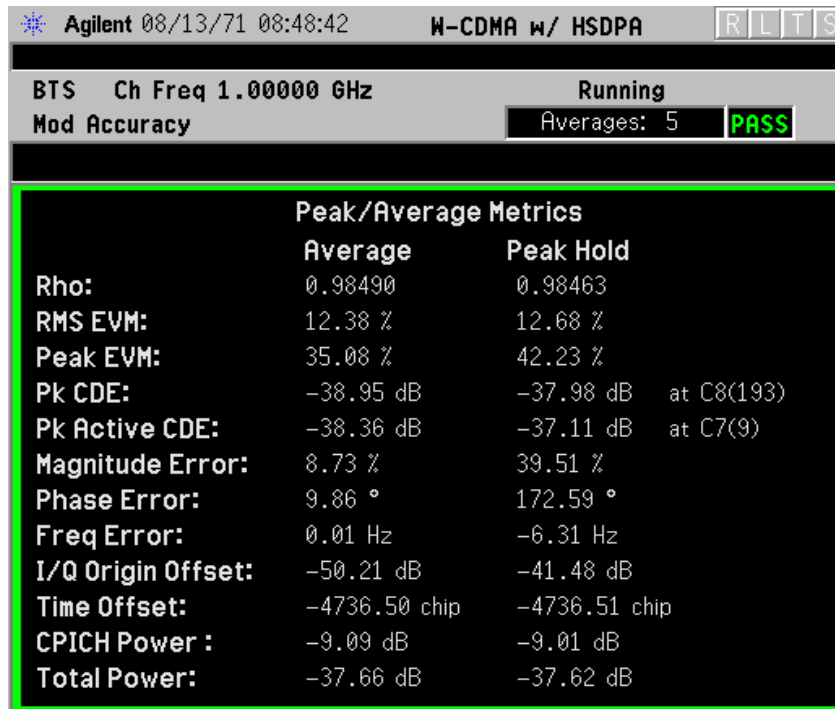
Figure 3-17 Mod Accuracy Measurement - Peak/Average Metrics View
